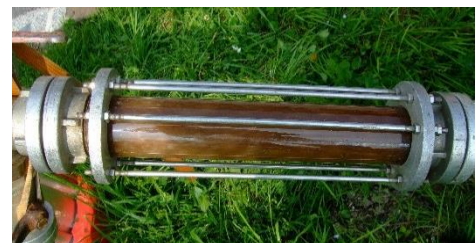
Figure 4: inspection glass during cleaning
