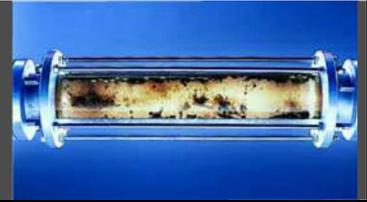
> We utilise the flowing water itself in the cleaning work by applying pressure to it – with “air scrapers”! With well-dosed, computer-calculated compressed air bubbles which we, carefully timed, inject into the water stream. This brings motion into play, leads to a high flow velocity, whirlpools and turbulences especially on the walls of the pipes. In doing so, the water sweeps the impurities away and finally transports them out of the system. >
