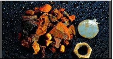
> The problem is as old as water supply itself. Even with the best water, there are impurities in the pipe system: floating, loose or muddy deposits, semi-solid incrustations as well as sand and stones. Microorganisms settle and biological films form on the walls of the pipes. The result: impurities and cloudiness. >
