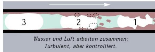
*The computer control takes into consideration all parameters which are typical for the location such as pipe diameter, flushing length, topography, operating pressure, standing pressure, impulse pressure and cleaning task.*
