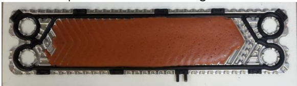
Fig. 9: Plate of heat exchanger with clay-gelatine-water deposit before cleaning
