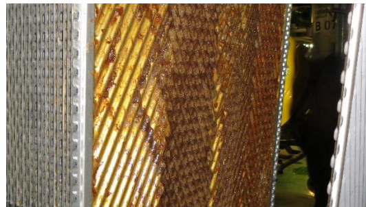
Fig. 16: Aged deposit after cleaning, model: mud from river water (Case from industry)
