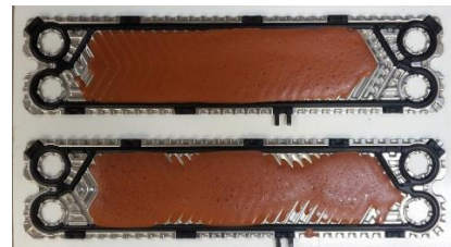
Fig. 6: Model deposit of clay, gelatine and water (Mud from rivers)
