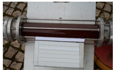
Figure 4: inspection glass during cleaning
