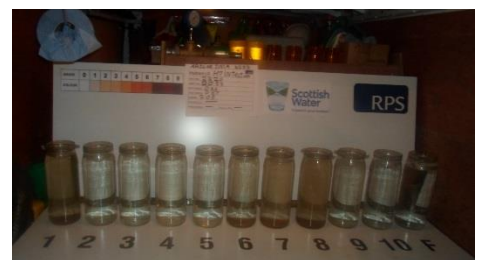
Figure 4: measurement of turbidity during cleaning
