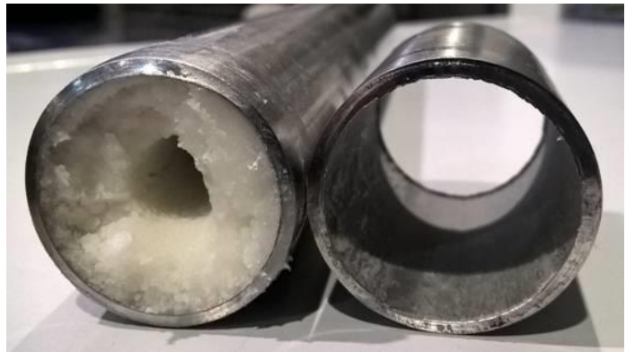
Figure 1: pipeline for cooling lubricant before cleaning (left side) and after cleaning (right side)
