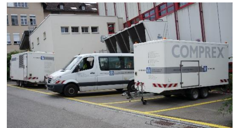
Figure 3: Comprex® unit on site
