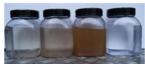
Figure 5: turbidity of rinse water during cleaning procedure
