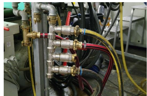
Figure 3: connection via adapters and distributor
