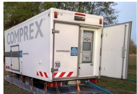
Figure 2: Controlling the cleaning impulses via Comprex® unit
