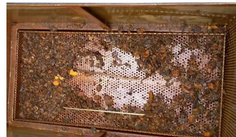
Figure 3: Large particle discharge from subsystem
