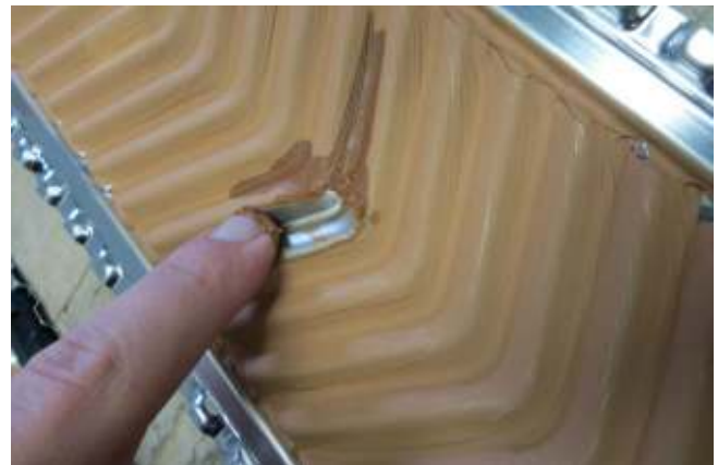
Fig. 8 Removal of model deposit by simple finger test.
