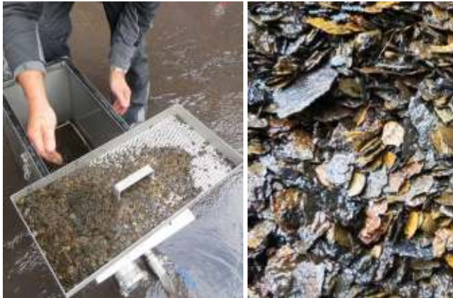
Fig. 16 Discharged fouling material in discharge unit (left) and in detail (right).
