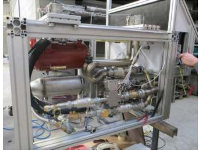
Fig. 7 Testing plant for cleaning plate heat exchangers.
