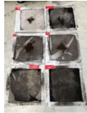
Fig. 4: Documentation of the particle discharge via filter fleece of 6 separate cooling circuits
