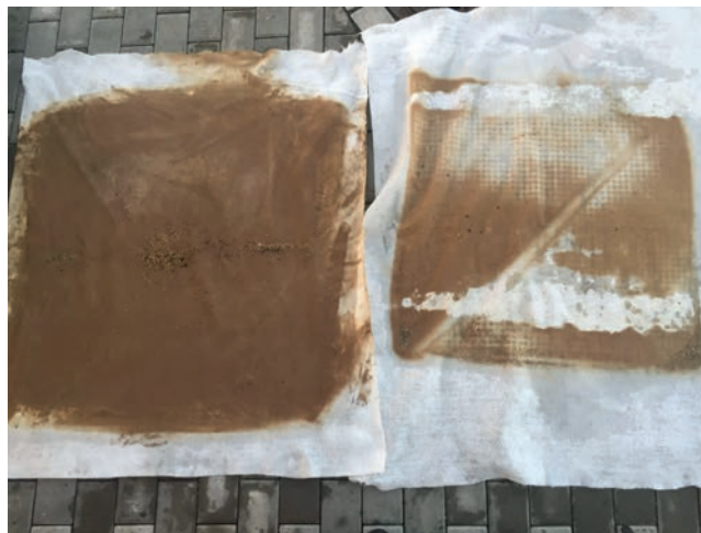
Fig. 4. Two filter fleeces loaded with removed particles. They can be disposed of without problems © Hammann
