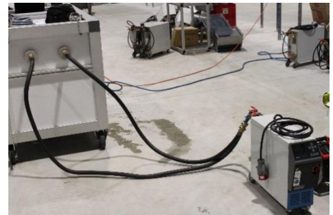
Figure 3: tempering unit during Complex® cleaning with MCE III
