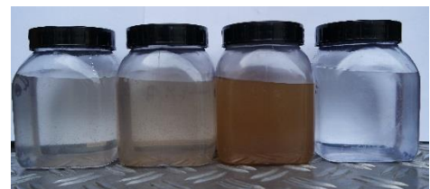
Figure 5: turbidity of rinse water during cleaning procedure
