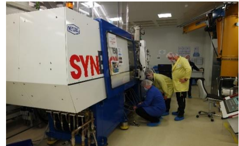
Figure 2: preparation of injection molding machines for cleaning
