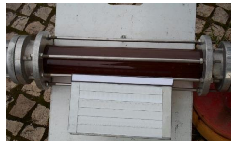
Figure 4: inspection glass during cleaning
