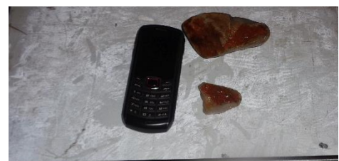
Figure 5: large particles removed from the pipe
