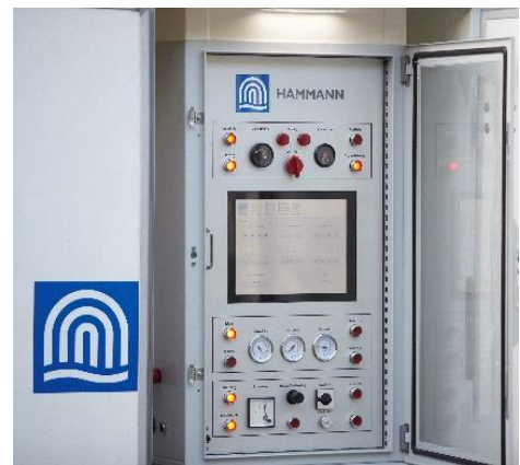
Figure 3: Impulse control system
