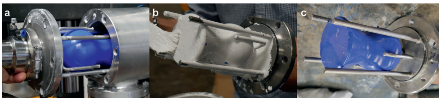
Figure 7: Pump with transparent plastic lid for tests after application of dispersion paint (left) and after cleaning (right). The QR code links to the corresponding video of the pump cleaning in real time.
