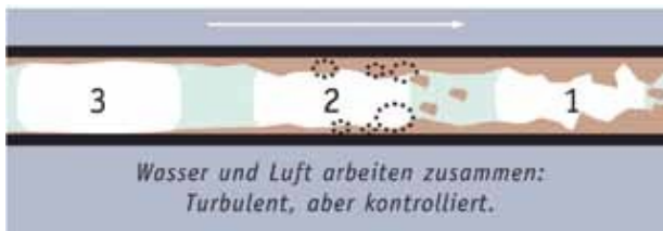
Fig. 5: Mobilizing the deposits with air and water blocks
