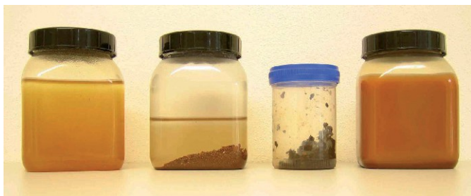
Picture 4 Discharges from drinking water installations in buildings
