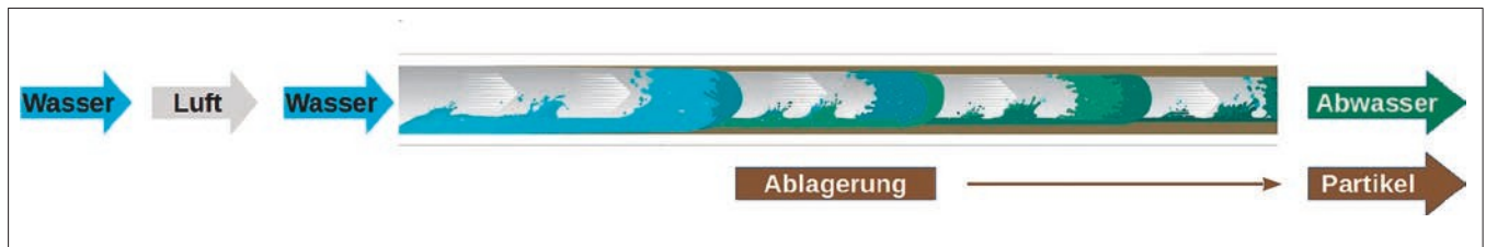
How Complex cleaning works: Alternating blocks of water and air remove impurities and deposits.
