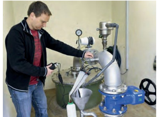
Figure 4: Faunistic sampling of the pipeline network. For this purpose, special nets are used to filter the largest possible volumes of water, usually 5 - 10 m 3 , and the animals contained therein are then sorted out, counted and determined. In addition, relevant water chemistry parameters are recorded.
