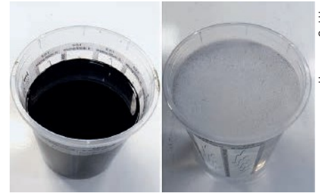
Fig. 6: Checking the success of cleaning. Pure acetone is poured into the charge air cooler and removed again after five minutes. Left: Contaminated solvent indicates an internally contaminated heat exchanger. Right: Clear solvent indicates an internally clean heat exchanger.
