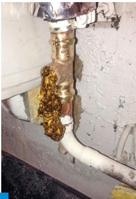
Discharge of a detached epoxy resin layer from a drinking water installation: there is no alternative to completely reinstalling the pipe system.
