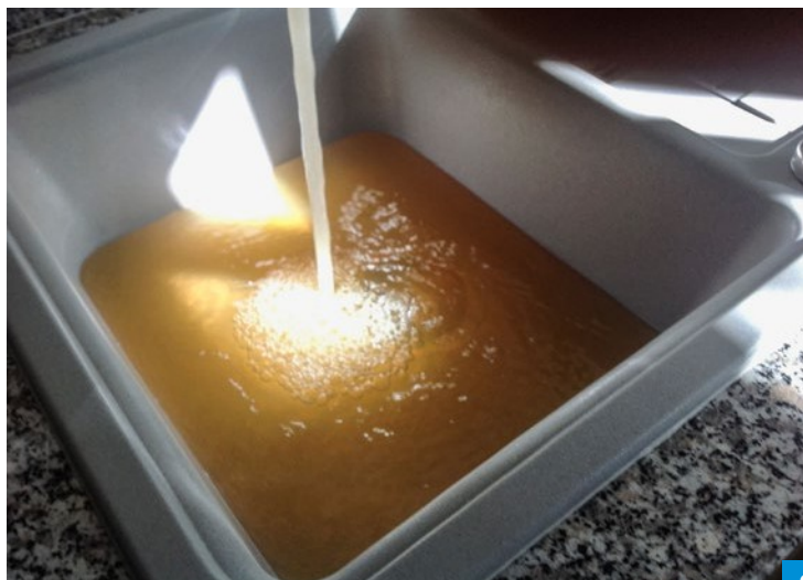
Corrosion in pipes made of hot-dip galvanized steel pipes often leads to considerable browning of the drinking water after thermal disinfection.
