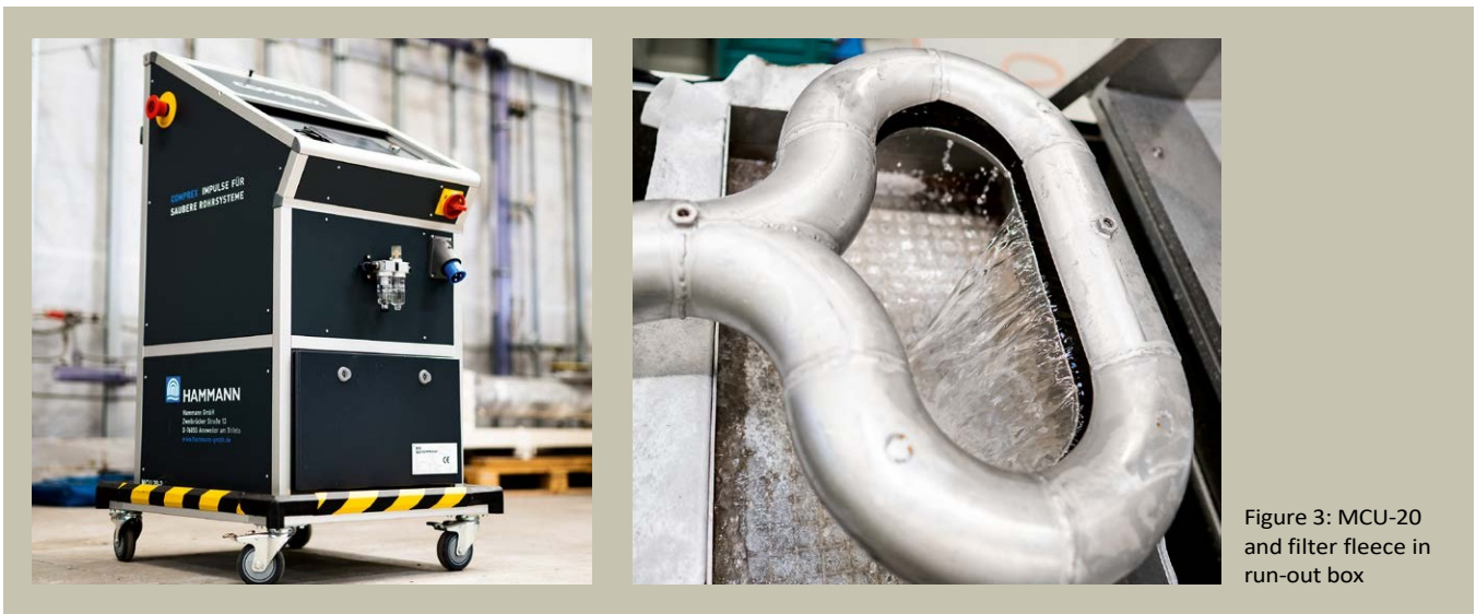
Figure 2: Discharge from the mold and machine circuits of the injection molding machines in the filter fleece of the Connect Box
