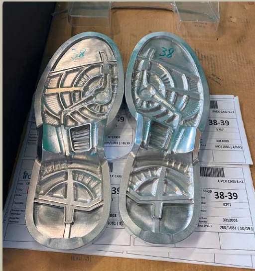
Figure 4: Example of injection mold and mold insert for shoe sole
