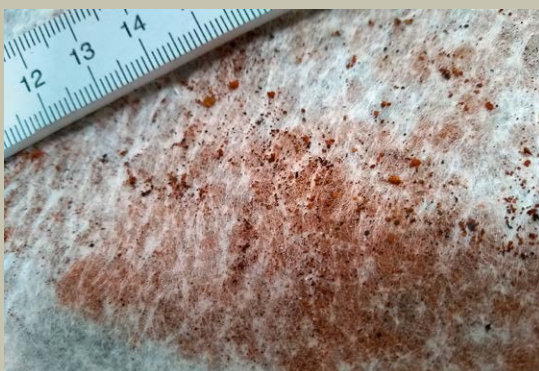
Figure 5: Discharged solids from injection mold on filter fleece
