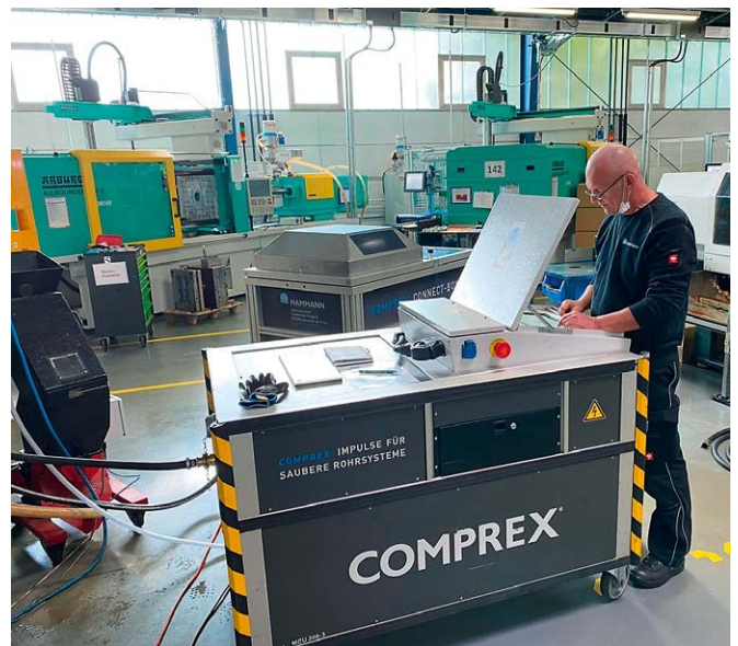
Image 1: MCU-300 during cleaning of the tool and machine circuits
