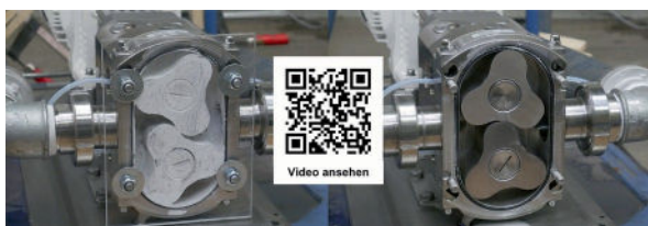
Fig. 9 // Pump with transparent plastic cover for the tests after application of the emulsion paint (left) and after cleaning (right). The QR code leads to the corresponding video of the pump cleaning in real time.
