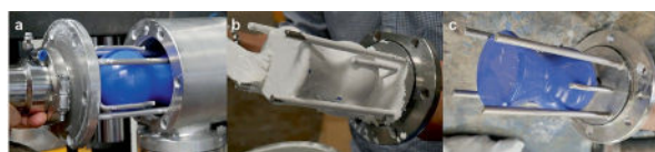
Fig. 8 // a) Pigging station, opened to remove the pig, b) Pig after application of the emulsion paint, c) Pig after cleaning.
