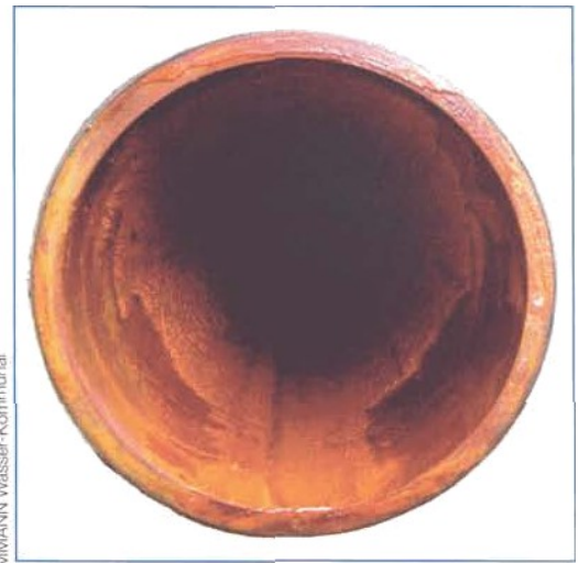
Fig. 13: Pipe section made of DN 350 AZ corrugation after successful pulse flushing
