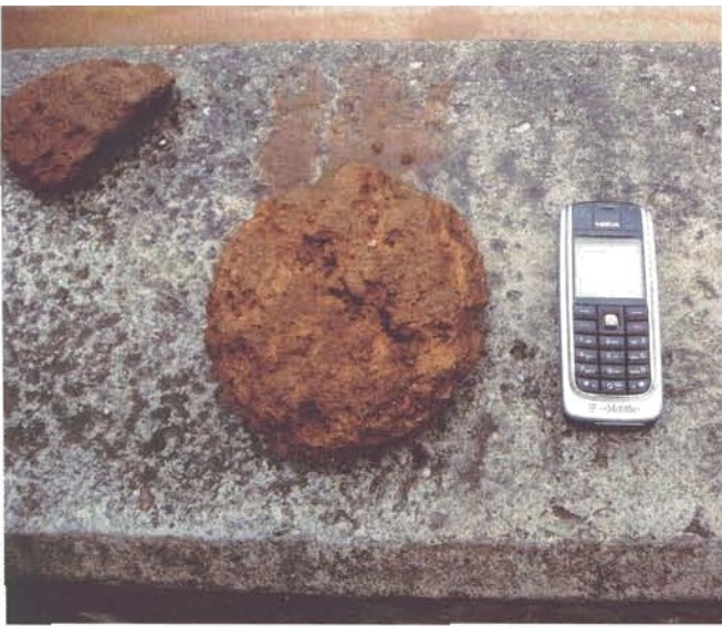
AbD. 12: Impulse flushing for AZ pipes with hard deposits: (a) Removal of hard deposits; (b) partially fossilized deposits
