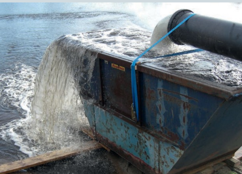
Figure 5: Feed-out during cleaning with the pulse flushing process
