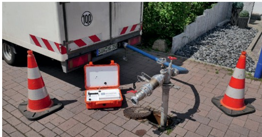
Fig. 11: Pressure measurement of a pipe section using a measuring box in practice
