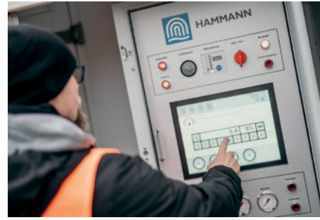
Fig. 3 Setting the cleaning parameters on the Complex trailer Source: Hammann GmbH
