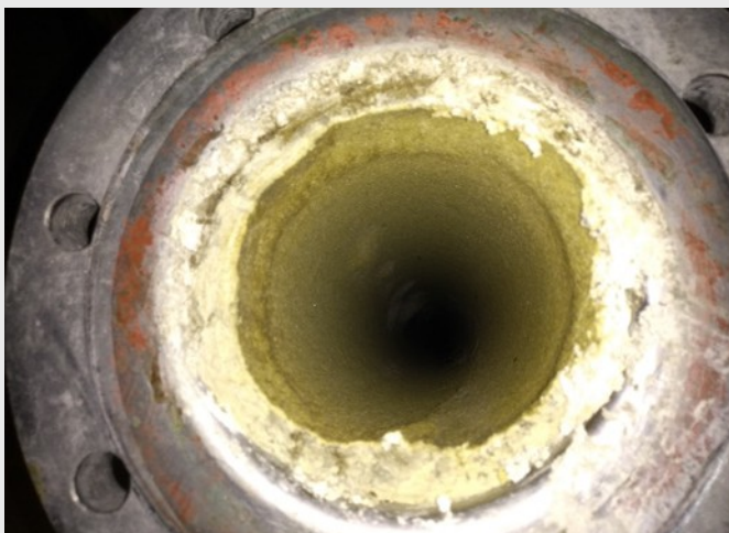
Figure 3: Deposits in the sludge pipe of a wastewater treatment plant and stationary Complex system
