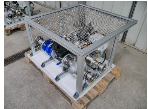
Figure 2: SCU as a wall module in the installed state with protective grille
