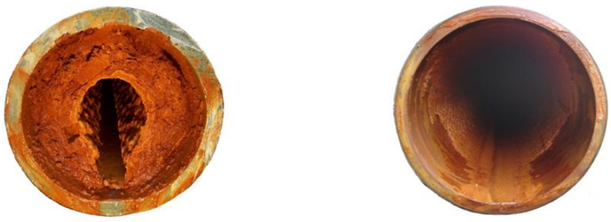
Figure 11: Raw water pipeline made of asbestos cement before and after comprex cleaning
